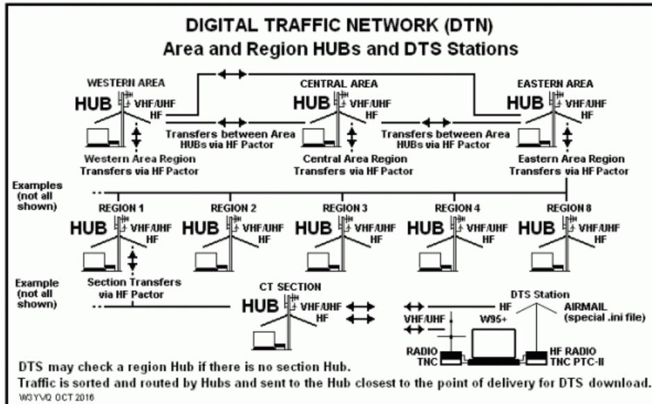
Figure 4: Digital Hub Operation
